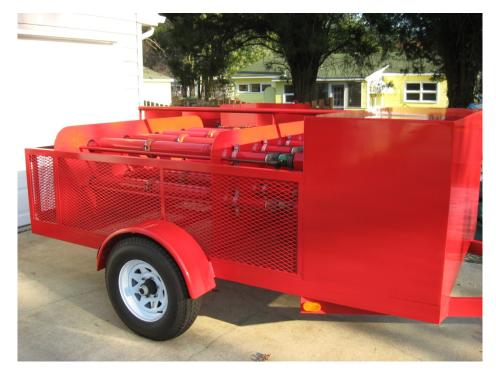
The EzFlow'n Unit can be custom built to flow whatever you request. Unit shown above is the 2000 Series able to flow up to 3750gpm
